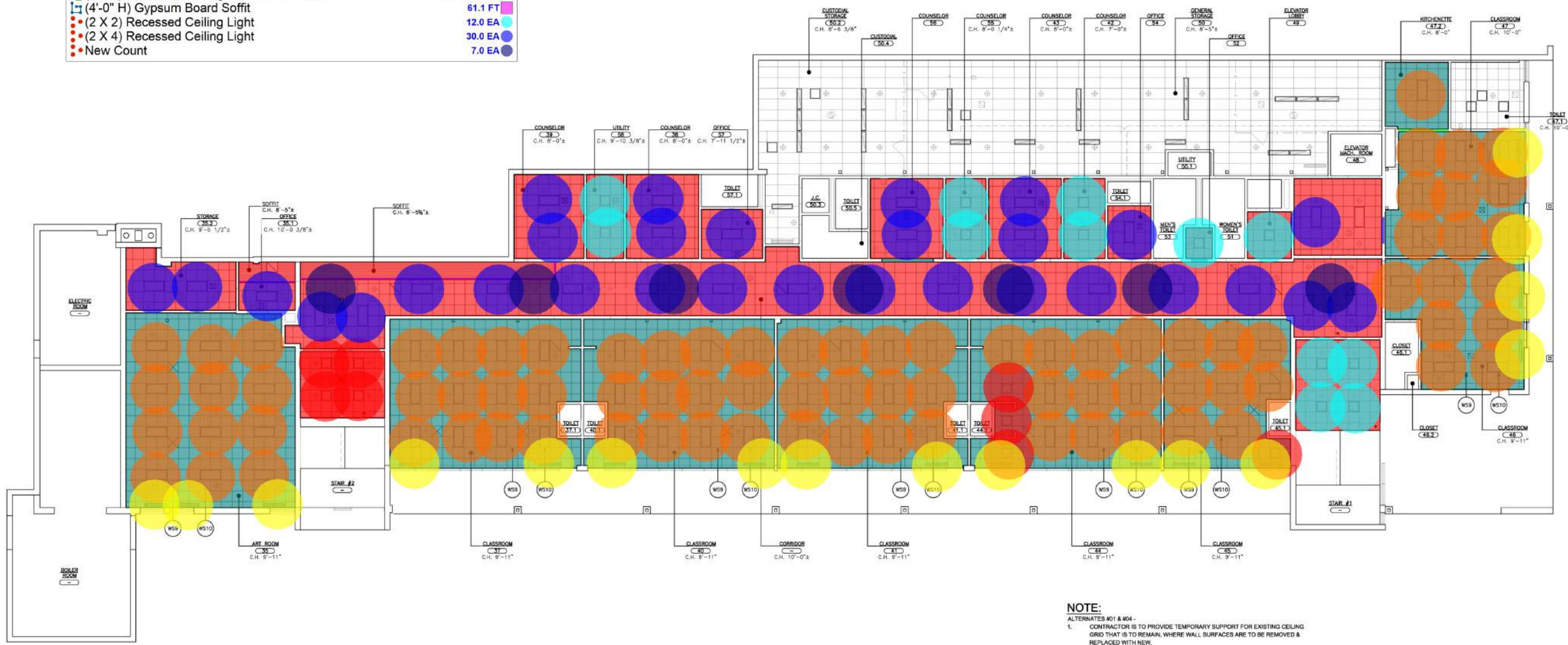
1 LOWER LEVEL REFLECTED CEILING PLAN - PROPOSED - ALTERNATES #02 & #05 SCALE: 1/8" = 1'-0"
